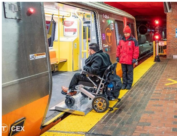
Photo 13: Bridge plate assistance
