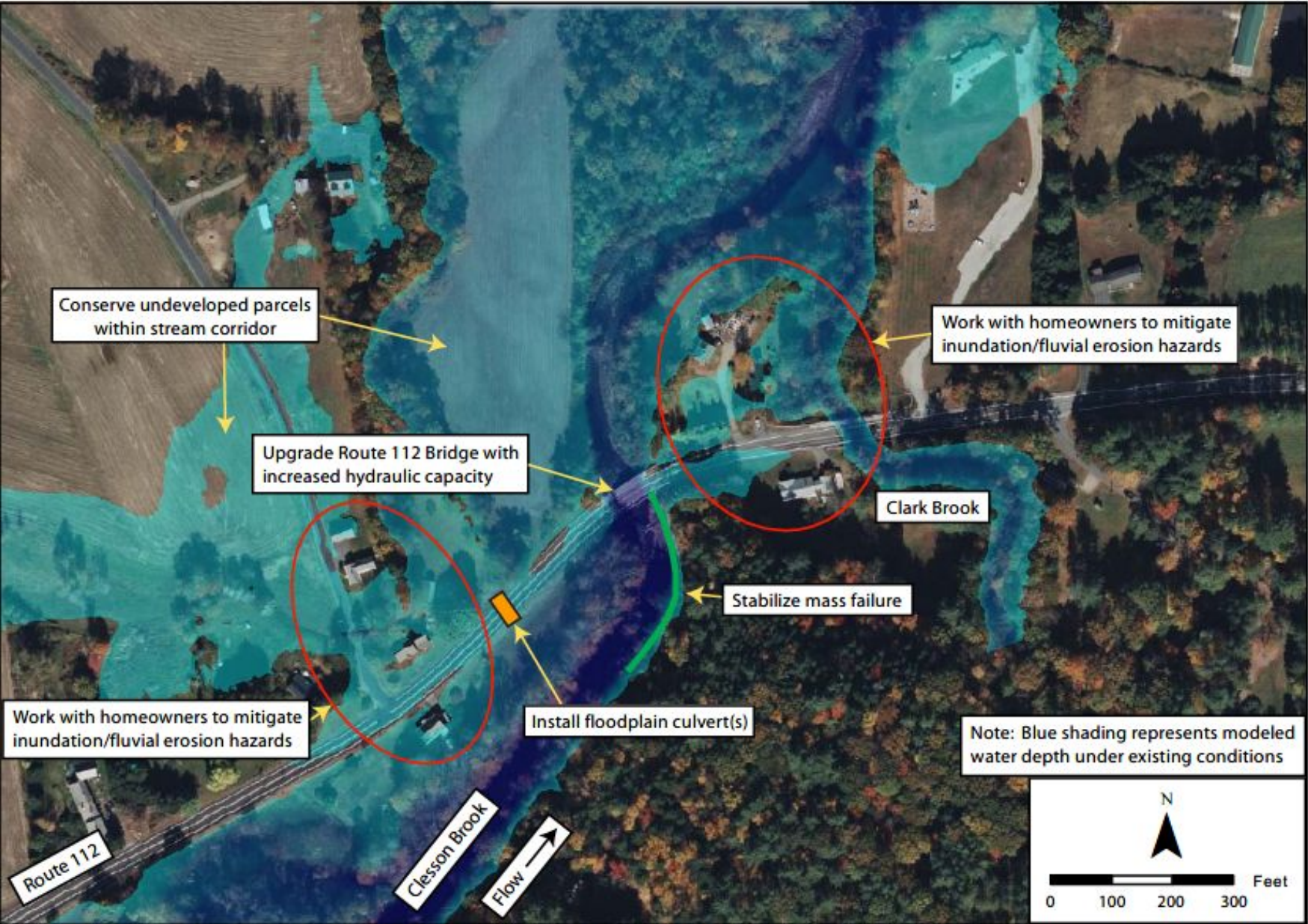
Clesson Brook - Route 112 Bridge Site (MassDOT B28004). Conceptual Design Plan View (Modeled Late Century 100-year flow event).
